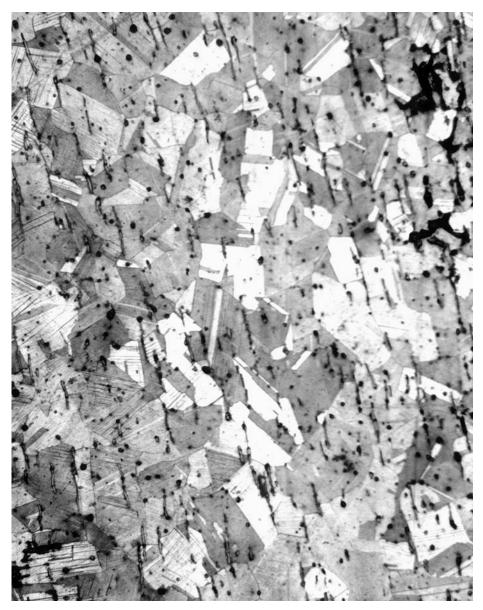
Fig. 9. Micrograph for the vessel (WK.A46-5) at a magnification of 200×, for a v-shaped section cut from the rim.
