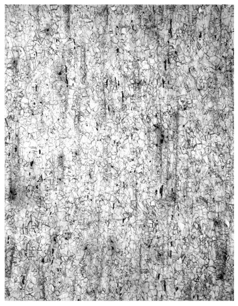
Fig. 11. Micrograph for the vessel (WK.B196-5) at a magnification of 200×, for a v-shaped section cut from the rim.
