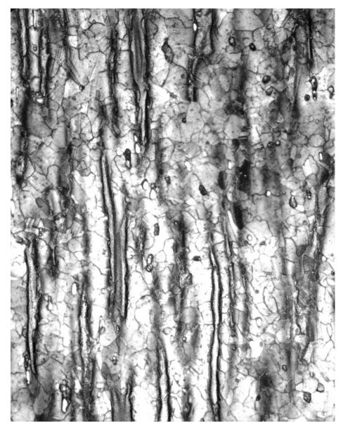
Fig. 12. Micrograph for the vessel (WK.B167-2) at a magnification of 600×, for a v-shaped section cut from the rim. Etchant: Klemm's III (Sn, 6.94%; As, 0.71%)
