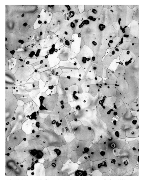
Fig. 15. Micrograph for the macehead (WK.B191-3) at a magnification of 200×, for a v-shaped section cut from the rim of the longer ferrule that is decorated with two circlets. Etchant: potassium bichromate + alcoholic ferric chloride (Sn, 6.7%; As, 0.35%)
