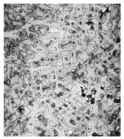
Fig. 18. Micrograph for the bell (inv. WK.A150-12: illustrated in plate 57,128) at a magnification of 200x, for a v-shaped section cut at the edge of the bell cavity. Etchant: ammonium hydroxide + hydrogen peroxide + alcoholic ferric chloride (Sn, 3.6%; As, 1.4%)
