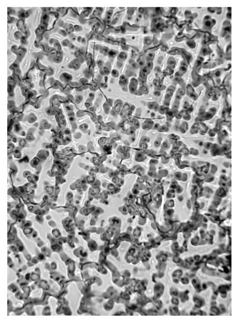
Fig. 16. Micrograph for the large button (WK.A150-5) at a magnification of 100×, for a v-shaped section cut from the edge. Etchant: ammonium hydroxide + hydrogen peroxide + alcoholic ferric chloride
