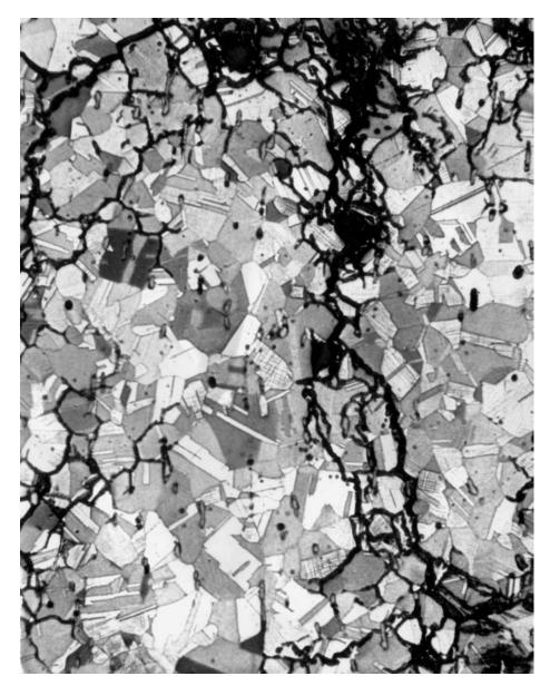
Fig. 10. Micrograph for the vessel (WK.A123-6) at a magnification of 200×, for a section cut off a fracture in the vessel's side wall, at the rim. Etchant: Klemm's III (Sn, 18.2%; As, 0.06%)
