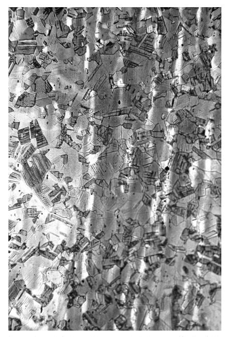
Fig. 17. Micrograph for the small button (WK.A150-9) at a magnification of 200×, for a v-shaped section cut from the rim.
