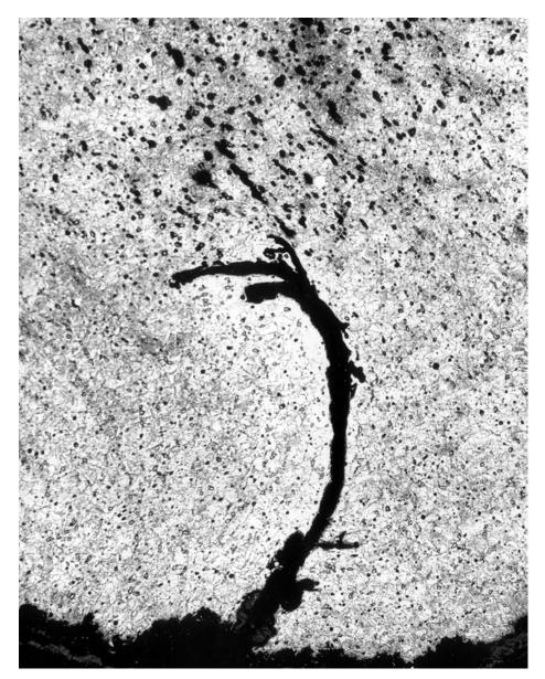
Fig. 8. Micrograph for the pin (WK.A22-3) at a magnification of 100×, for a cross-section cut from midway down the shaft, where the tip is broken off. Etchant: potassium bichromate + alcoholic ferric chloride (Sn, 9.0%; As, 0.33%)
