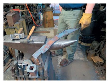
FIGURE 12 The replica *kopis*, after three cycles of heating in the forge and hammering (Author's photo).
