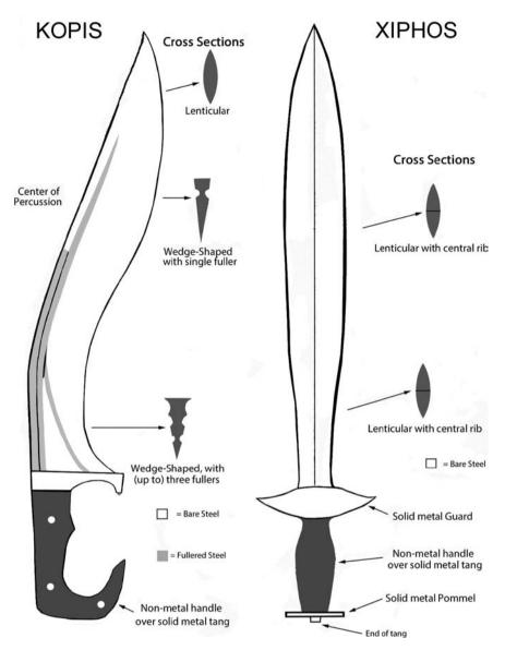
FIGURE 1 Drawn diagrams of a typical (Verčík Type 4) kopis and a typical xiphos with crosssections of the blades. (Author's drawing).
