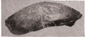
2. PLATE GIVING FIRST CURVATURE. CHALKLINE DENOTES FUTURE CREST
