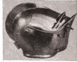
17. FILED AND POLISHED, BORDERS FINISHED, BANDS READY FOR DECORATION
